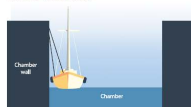
Small craft is positioned and tied sidewall
