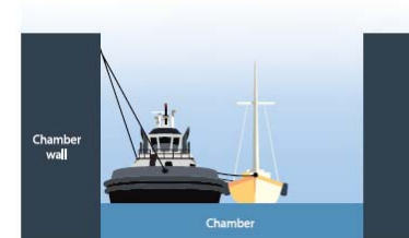
Small craft is positioned and tied at the side of a Panama Canal Tug
