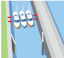
1 Small crafts approaches the chamber tied up with required fenders at sides (and between them)
