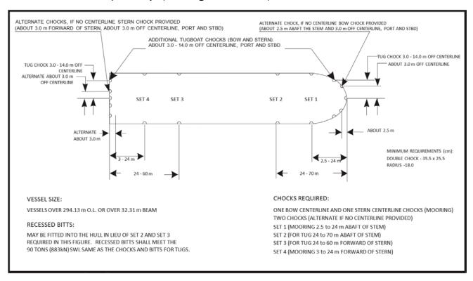
FIGURE 7 – Location of Chocks and Bitts (Neopanamax and Panamax Plus)
