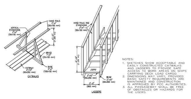
FIGURE 5 - Catwalk and Ladder Sketches
