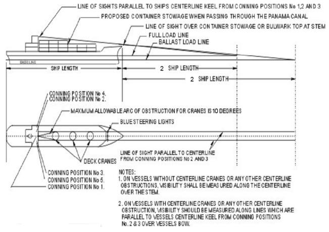
FIGURE 4 - Normal Conning Positions
