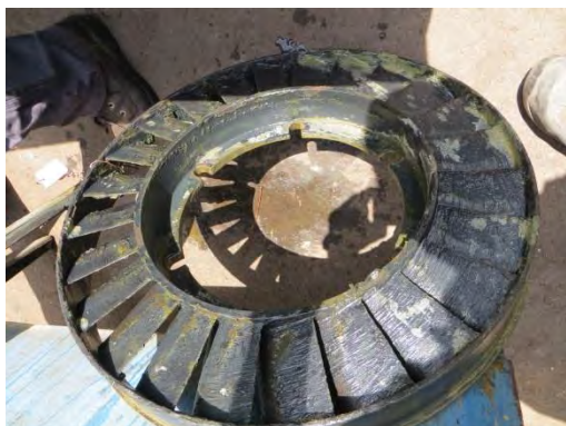
Nozzle ring before cleaning
