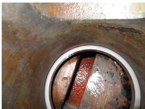
The grey ring is the landing surface for the exhaust valve cage.
