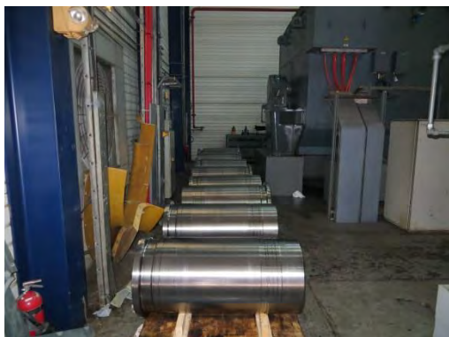
New liners ready for installation.
