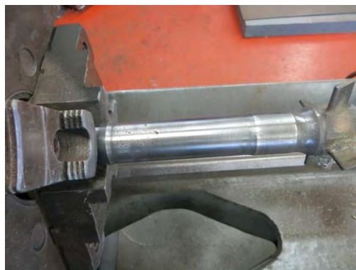
Exhaust valve with pitting markings
