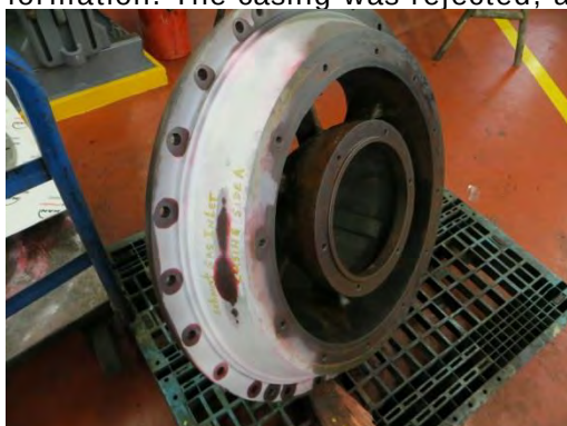
T/C "A" gas admission casing
