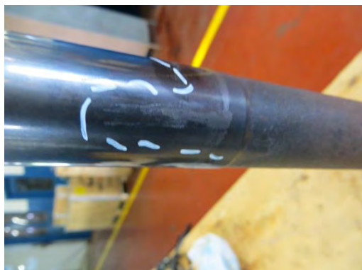
Exhaust valve with scuffing markings
