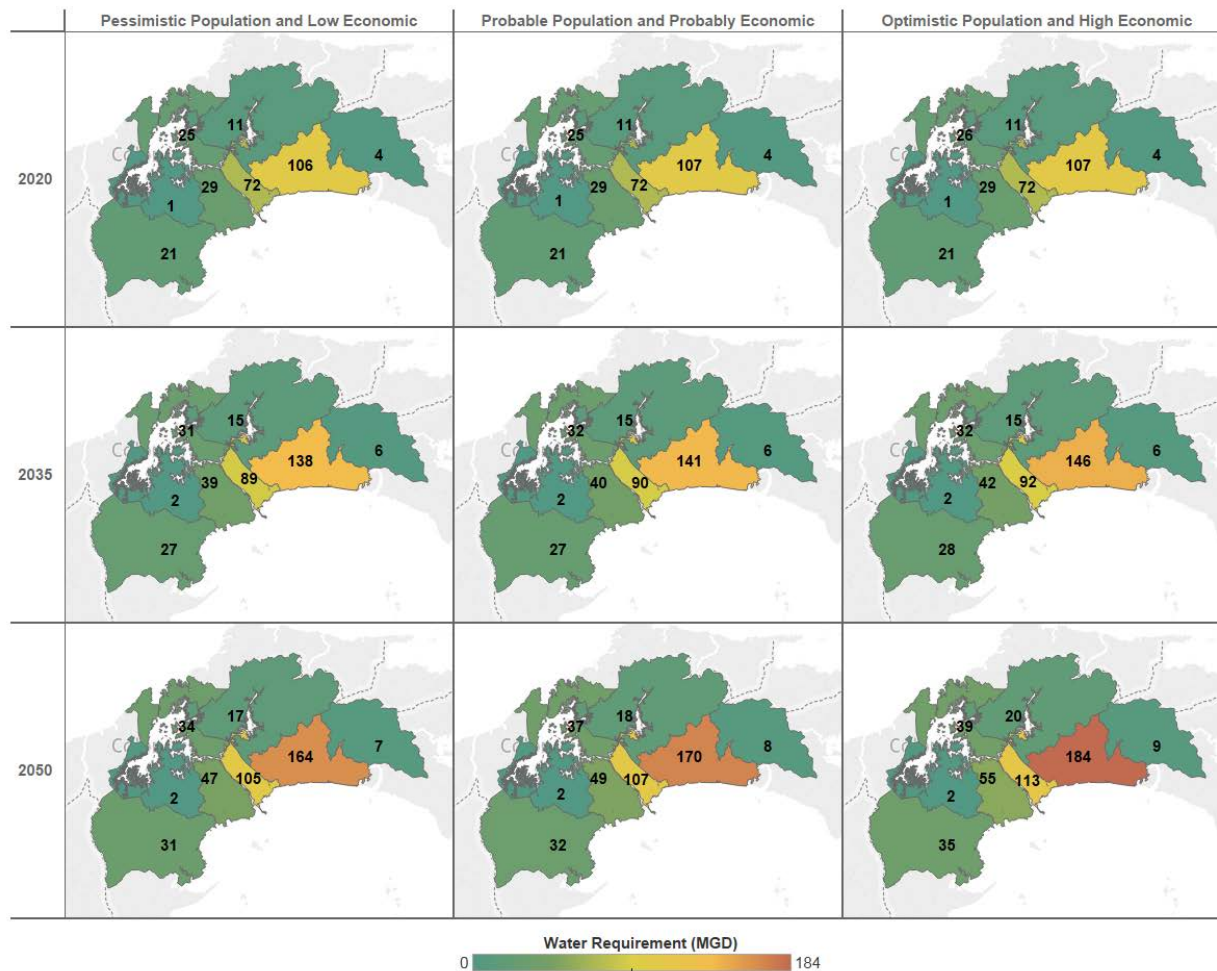
Figure 5.20 – Population Zone map of forecasted total water requirement at select future years and population/economic growth projection combinations for Minimum Requirement scenario
