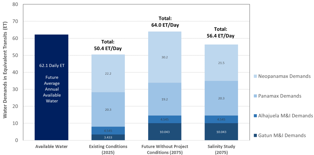
Figure 5-5: Water Demand for Existing Conditions, Future Without Project Conditions, and the Expected Results from the Salinity Study
