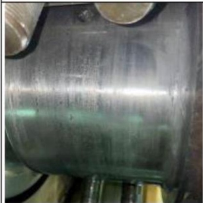
Main Journal from unit #1 as found. Its recommend to remove the complete crankshaft for engine frame housing evaluation.
