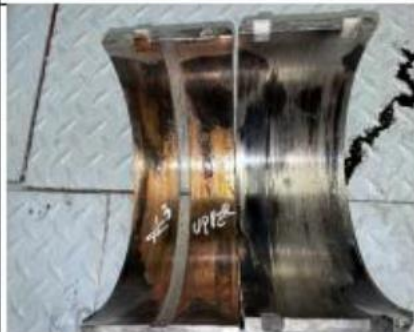
Bearing shells from unit #3 from the main journal.
