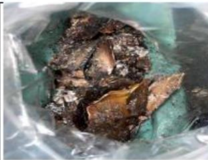
Metal particles found in the crankcase during the incident.
