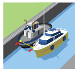
2 Small craft is tied up to the Tug, which is positioned at the side of the wall
