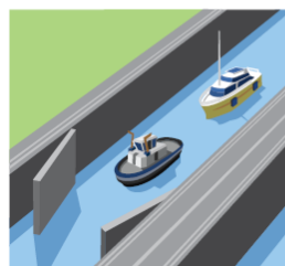
1 Small craft approaches the chamber behind the Tug and with required fenders
