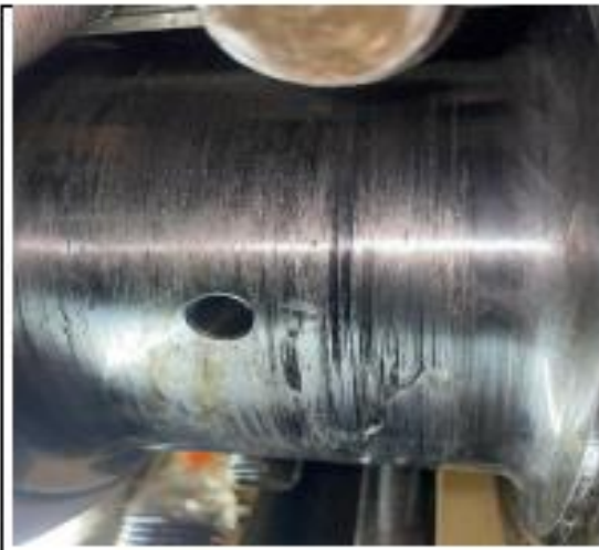
Main Journal as found from unit #3 inspected during our inspection.
