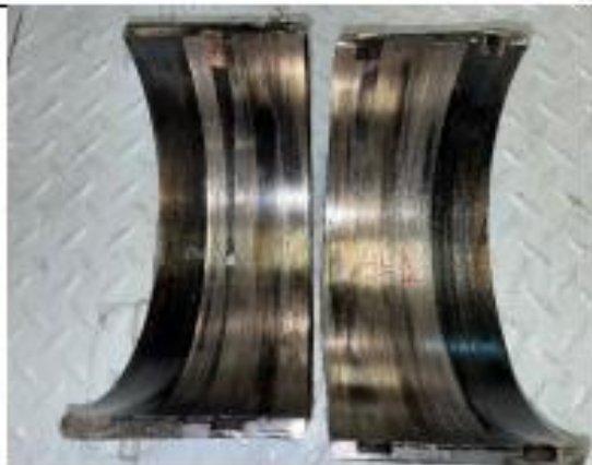
Bearing shells from unit #1 as found during our visit.
